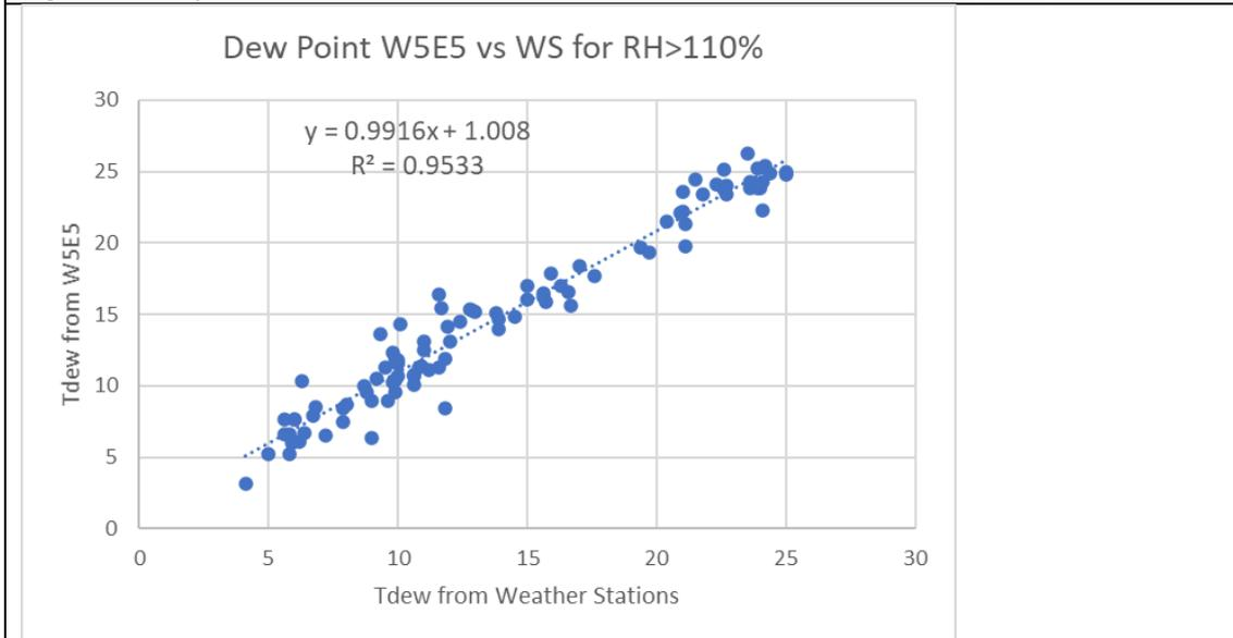
**Figure 2** Comparison of weather station Tdew with W5E5 Tdew where RH(Tmin)> 110%
